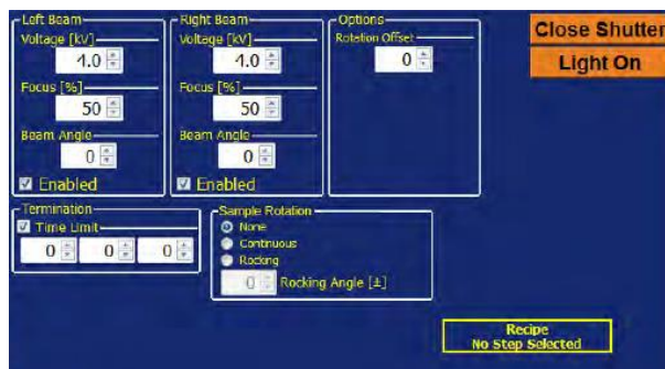
Figure 2. Milling Commands for sample processing.
